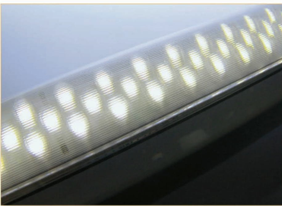
The LED tubes which are new and saving energy up to 80% have 396 LED at the 150 cm LED tubes. This guarantees an even, balanced luminance. (Photo: Markus Frutig, elFORUM)
